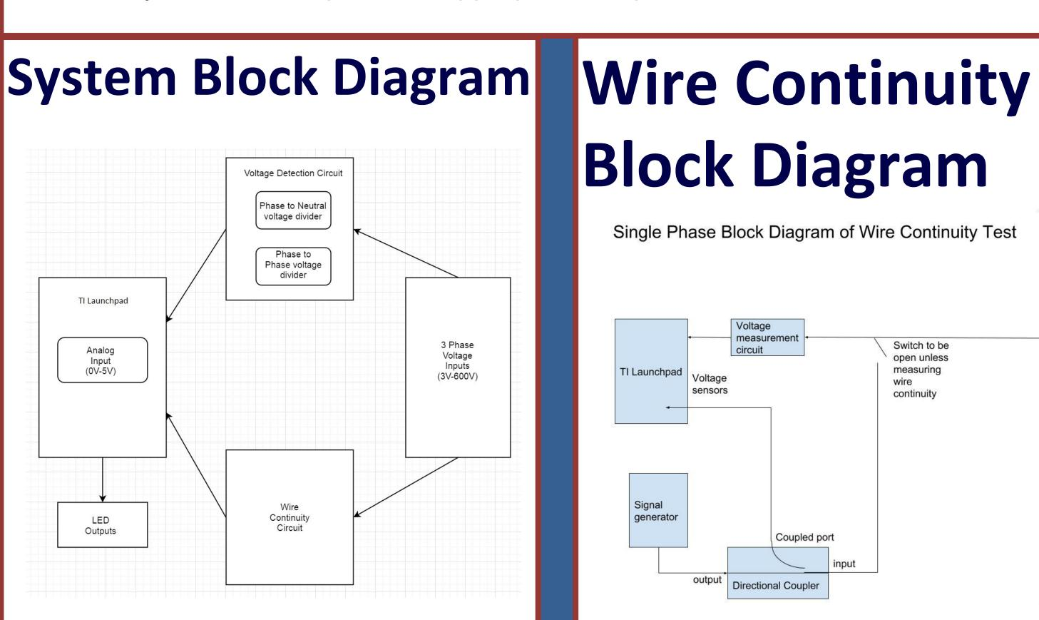
reflection of the sine wave will be coupled and sent to TI Launchpad to be measured and analysed
